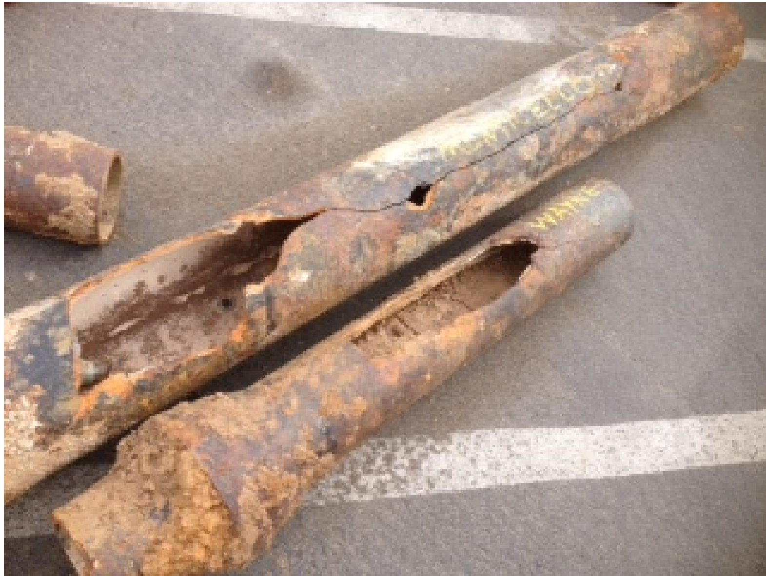
Failed Cast Iron Distribution mains removed from service December 2014. Installed c. 1950.
