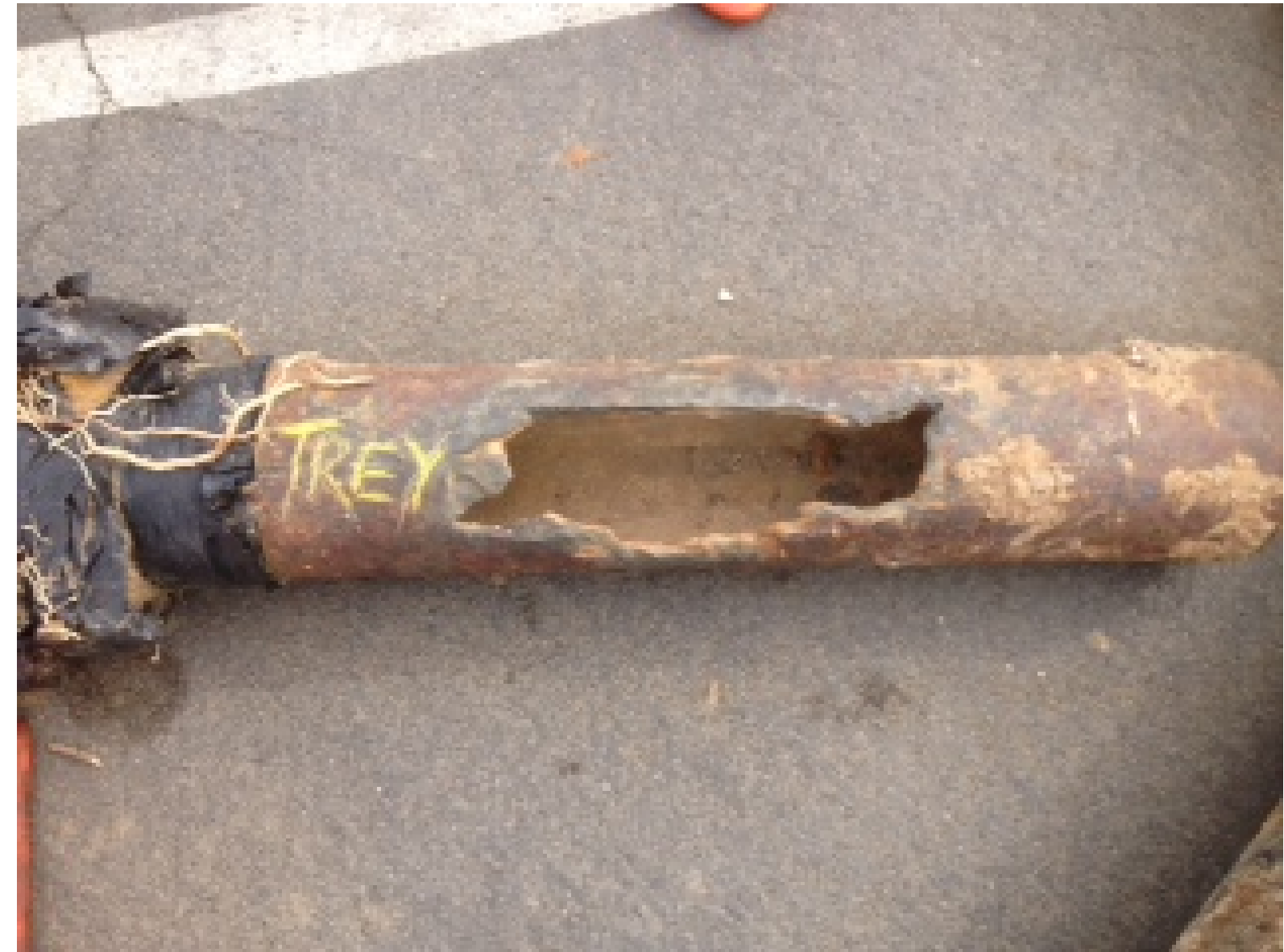
Failed Cast Iron Distribution mains removed from service December 2014. Installed c. 1950.
