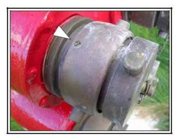
6. Remove the set screw, keeping the bearing opening upward so as not to lose the ball bearings.
