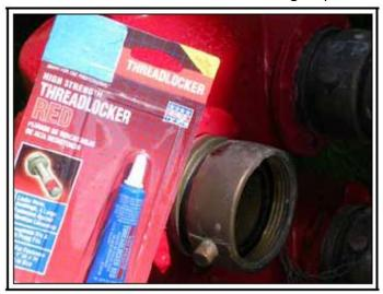
Tape helps to hold the set screw on its side, while applying thread locker
