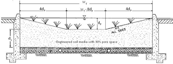
a. For the design with side slopes the following equation shall be used to determine the total effective depth. Where,  $d_P$  is the depth of ponding within the basin.
