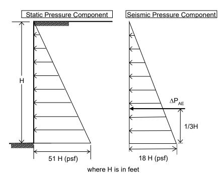
Seismic Earth Pressure Distribution on Walls
