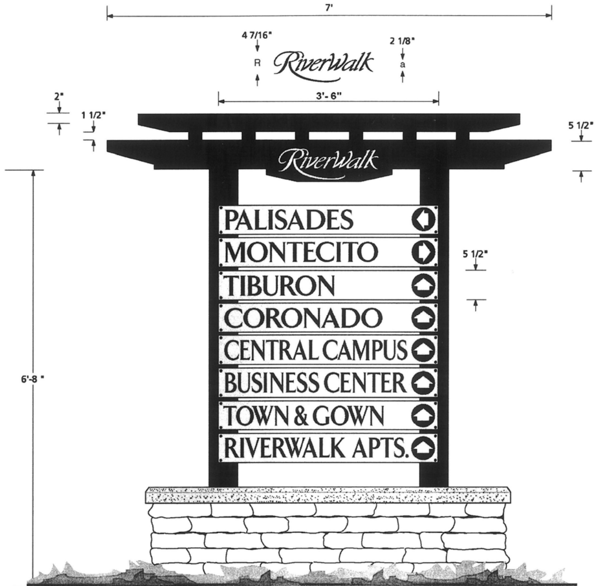
S/F KIOSK STRUCTURE W/ RE-SAWN HEADER, POSTS AND TRELIS, ROUTED LOGO TYPE AND ATTACHED ALUMINUM 1/8" PAINTED AND VINYL COPY RIDERS
