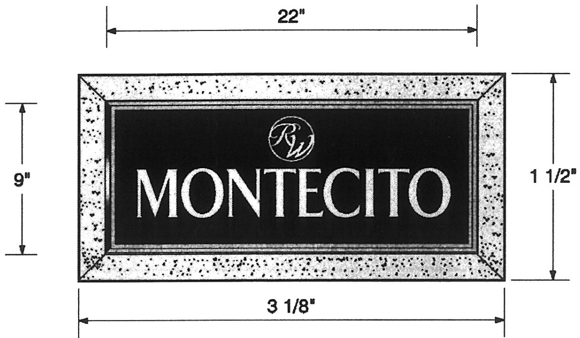
3/8" CASTED BRONZE PLAQUE MOUNTED IN CASTED CEMENT FRAME WALL PLACEMENT TO BE DETERMINED
